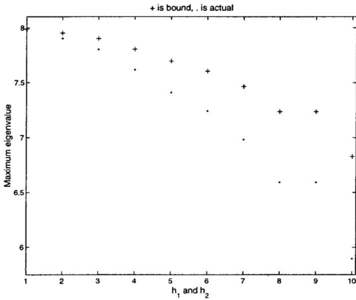
FIG. 2. Maximum eigenvalues of  $A^{(2)}(40^2, \sqrt{2k^2})$  for the directions  $h_1 = \pm k$  and  $h_2 = \pm k$ ,  $k = 1, \dots, 10$ . The actual maximum eigenvalues are given under each bound, and the bounds  $2\lambda_{max}$  are labeled by +. The bound becomes worse as  $h$  increases.
